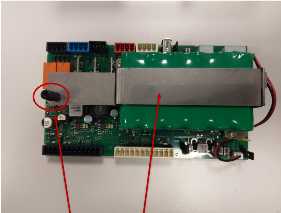
Remove the spacer screw and the fixing plate.
