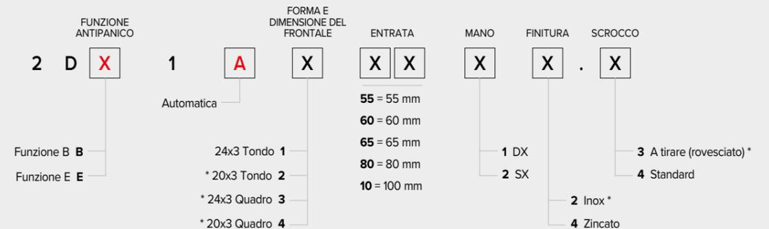
CONFORME ALLE NORME DIN 18251 - EN 12209 - EN179 - EN1125
